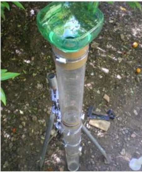
Twenty BEST infiltration experiments at randomly selected points within a 150 m 2 area
