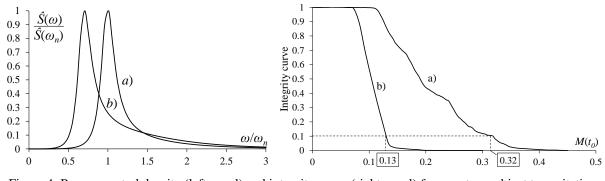
Figure 4: Power spectral density (left panel) and integrity curve (right panel) for a system subject to excitations having spectral parameters: a)  $k_1$ =0.97,  $c_1$ =0.2,  $k_2$ =3.44,  $c_2$ =2.32; b)  $k_1$ =0.47,  $c_1$ =0.2,  $k_2$ =3.44,  $c_2$ =2.32.
