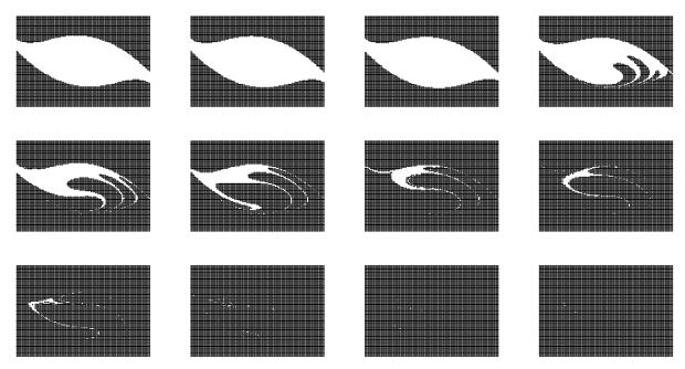
Figure 3: Safe basins obtained by increasing values of  $M(t_0)$ , uniformly distributed over the interval [0,0.45].
