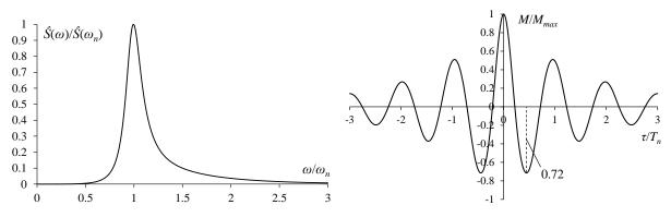
Figure 1: Quasi-deterministic representation of the exciting moment M(t) with spectral parameters:  $k_1$ =0.97;  $c_1$ =0.2;  $k_2$ =3.44;  $c_2$ =2.32. Left panel: power spectral density. Right panel: time variation of the excitation.
